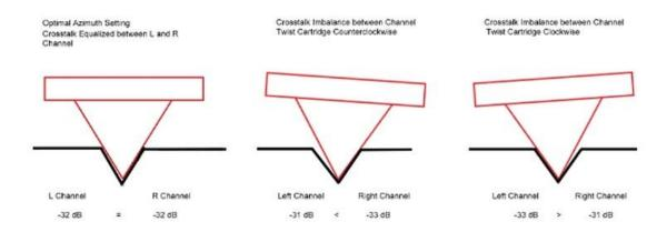
The AnalogMagik software and test LP contains two test tracks which all allow you to determine the level of crosstalk between two channels. To determine the optimal azimuth, take readings of the two Azimuth tracks on the test LP, and AnalogMagick will compute the Crosstalk number for you.
