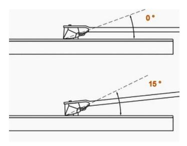
The Acoustical System <u>SMARTstylus</u> is an excellent tool which will allow you to visually gauge an initial Stylus Raking Angle. The Uni-Scope
