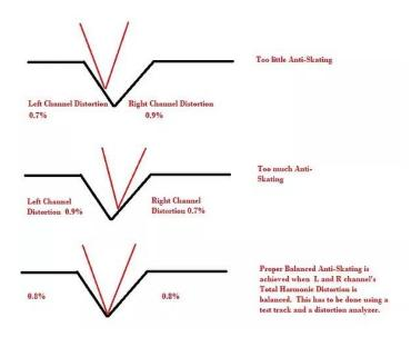
Play the anti-skating test track on the AnalogMagik Test LP, and use the Anti-Skating function on the AnalogMagik software. Repeat the measurements with increased or decreased anti-skating force.. The anti-skating force is optimized when the distortion figures between the Left and the Right channel is balanced or as close together as possible. We also
